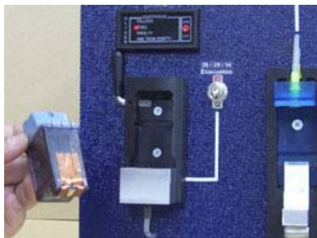
Check, if the cartridge is undamaged for filling
